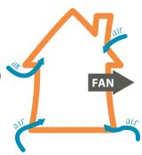
building cavities. A difficulty with exhaust-only ventilation is the inability to control where the outside air is being pulled from. In humid climates, however, this ventilation strategy can lead to significant moisture problems.
