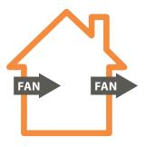
Heat Recovery Ventilators (HRVs) are installed to achieve the balanced flow and work well with non-traditional systems, such as mini-split HVAC systems and ground-source geothermal systems. This ventilation strategy can be used in any type of climate, but is highly recommended for costal and marine areas.
